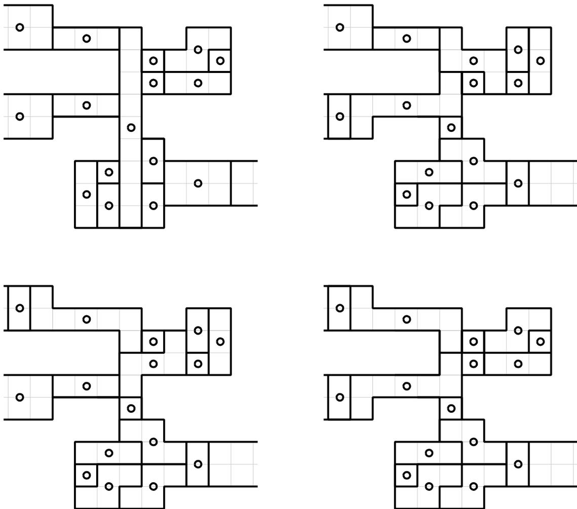
Figure 6. The four possible states of the AND gate
