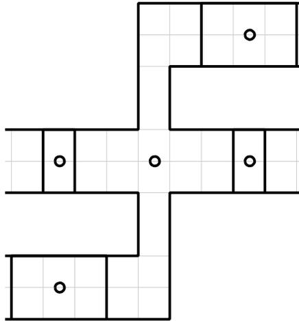
Figure 7. A TRUE signal crossing a FALSE signal
